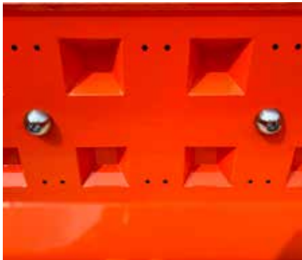
1 Place the magnets in the center of the concrete mould.
