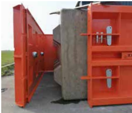
4 When the mould is opened, the magnet remains in the mould.
