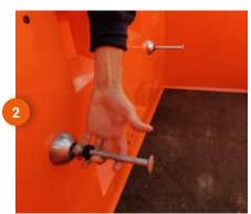
Place the rubber around the anchor, place the anchor in the magnet
