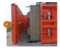
When the mould is opened, the magnet remains in the mould
